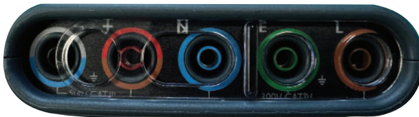
Fig.2 Interlock in position for RCD & Loop testing
