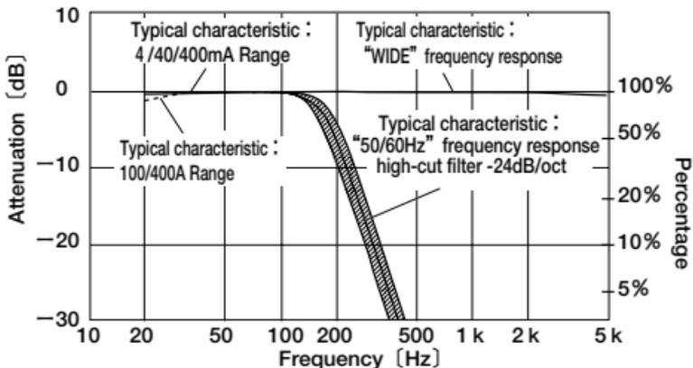
Fig.3 Model 2432/2433 Frequency Characteristic
